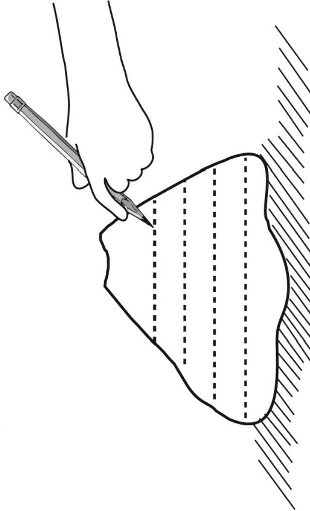
**Step 5: Slice the model to create contour lines.**
